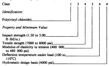
Note 3—The cell-type format provides the means for classification and close characterization and specification of material properties, alone or in combination, for a broad range of materials. This type format, however, is
